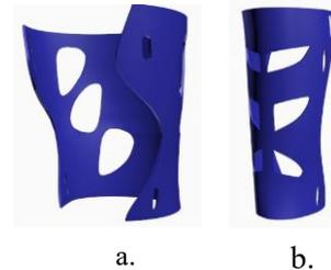
Figure 1: 3D models of (a) hip and (b) leg brace based on geometry of 7 year old child.
